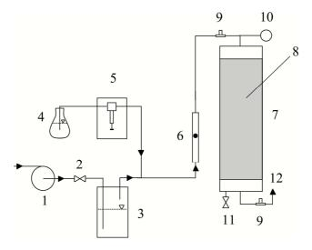
Figure 1 - Experimental set-up of biofilter system. 1 - blower, 2 - needle valve for flow rate control, 3 - humidification vessel, 4 - vessel with toluene and xylene, 5 - syringe pump, 6 rotameter, 7 - biofilter, 8 - packing, 9 - sampling ports, 10 - manometer, 11 - valve for leachate, 12 - outlet
