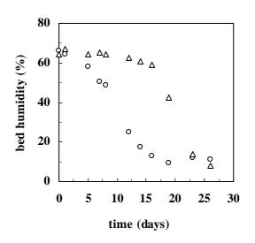
Figure 3 - Drying out of the packing at different air flow rates.  $\circ$  - air flow rate of 1 L.min<sup>-1</sup>  $\Delta$  - air flow rate of 0.5 L.min<sup>-1</sup>
