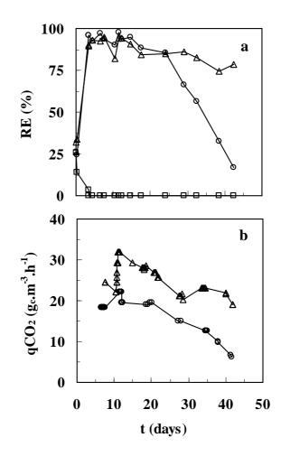
Figure 2 - Comparison of performance characteristics for the different biocatalysts. a - Removal efficiency, b - CO<sub>2</sub> evolution rates  $\Box$  - sterilized biofilter,  $\circ$  - uninoculated biofilter,  $\Delta$  - inoculated biofilter
