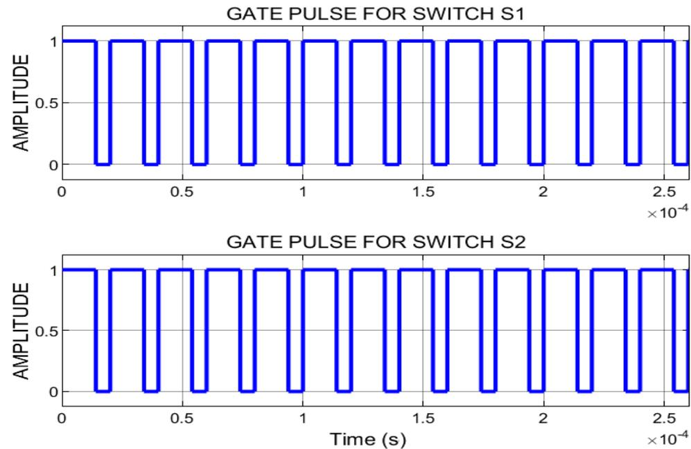
**Figure 7.** Gate pulse waveforms for the switches  $S_1$  and  $S_2$
