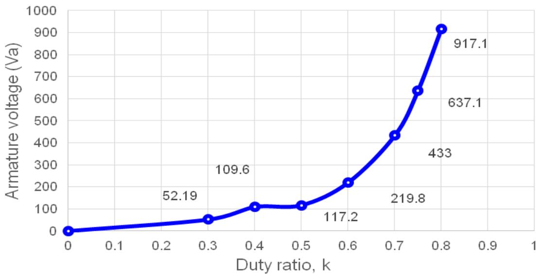
**Figure 13.** Variation of motor armature voltage with duty ratio (k)
