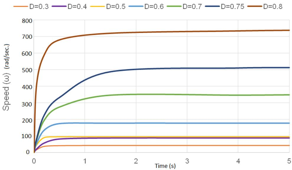
**Figure 10.** Variation of motor speed (rad/sec) with duty ratio (k)
