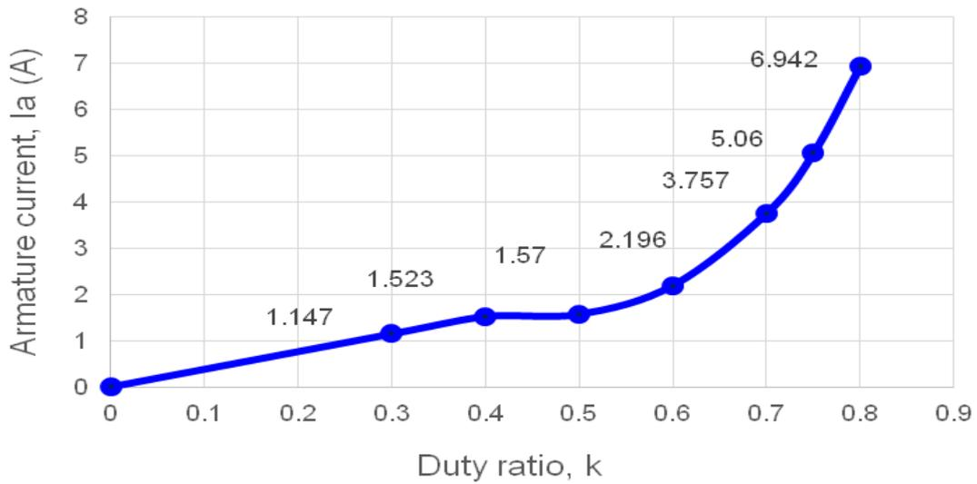
**Figure 12.** Variation of motor armature current with duty ratio (k)
