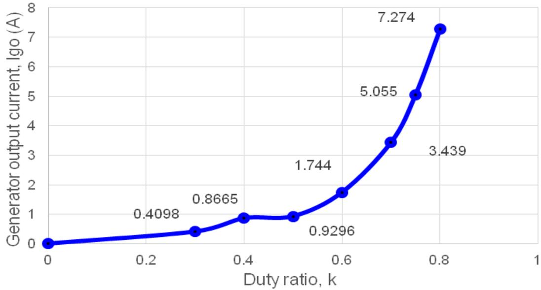
Figure 14. Variation of generator load current with duty ratio (k)
