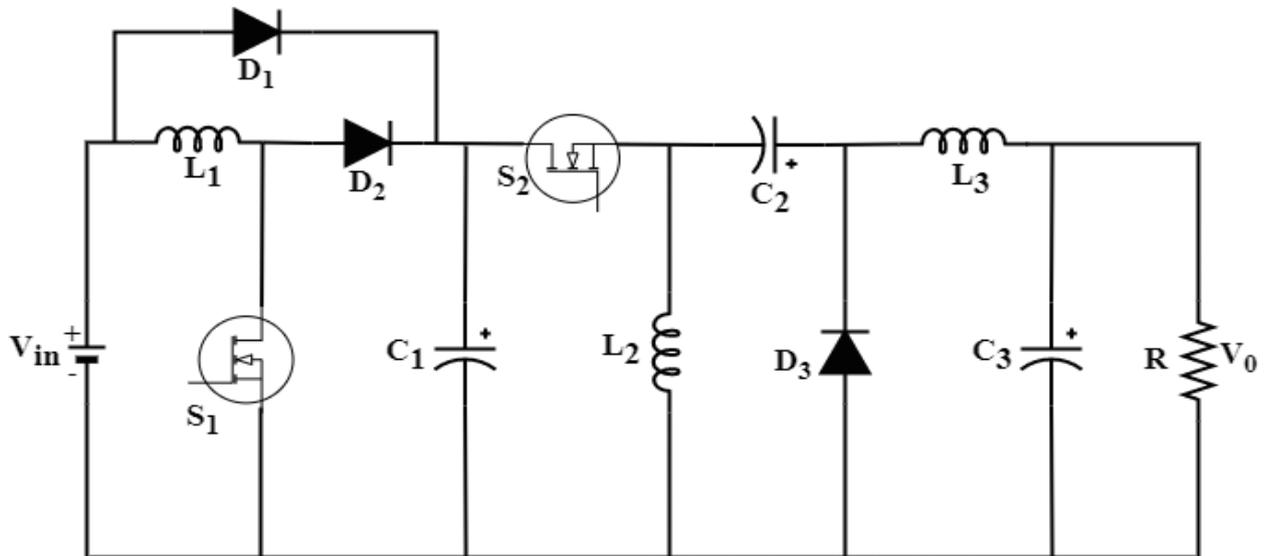
**Figure 1.** Power circuit diagram of Zeta converter-fed Separately excited DC motor coupled with DC generator
