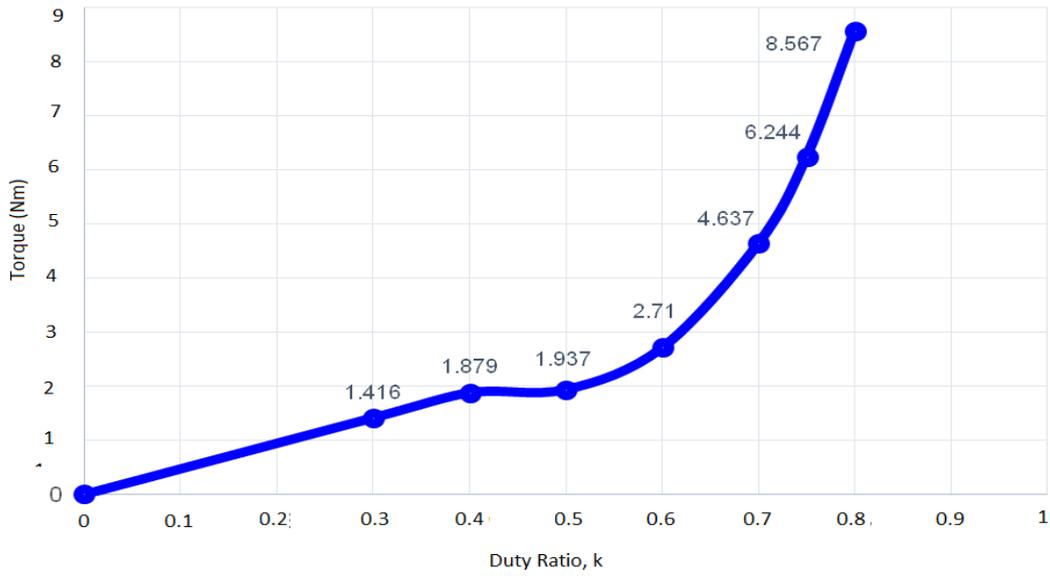
**Figure 11.** Variation of motor torque (Nm) with duty ratio (k)
