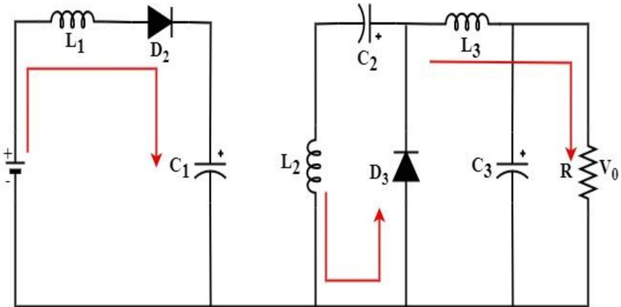
Figure 3. Equivalent circuit of the converter during Mode-II
