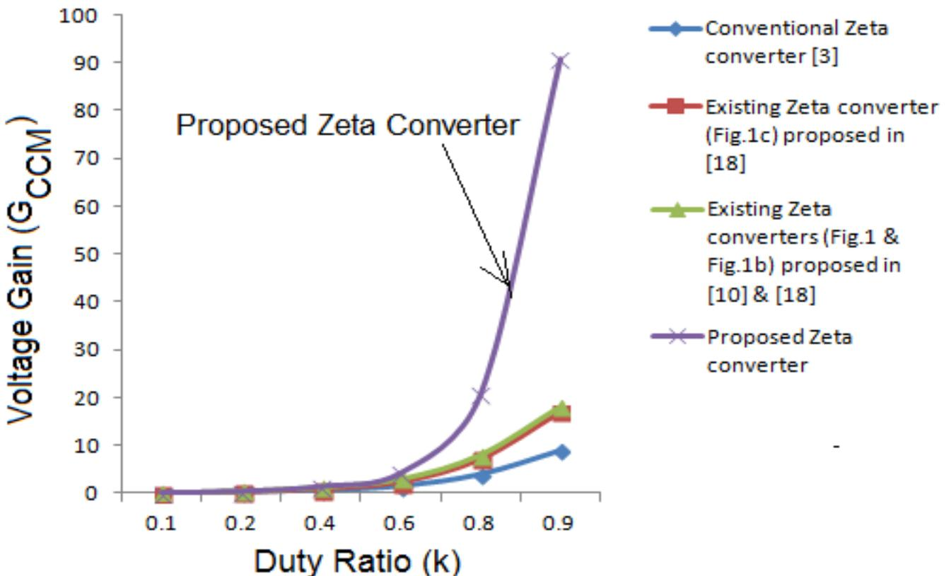
Figure 5. Comparison of proposed Zeta converter with other Zeta topologies
