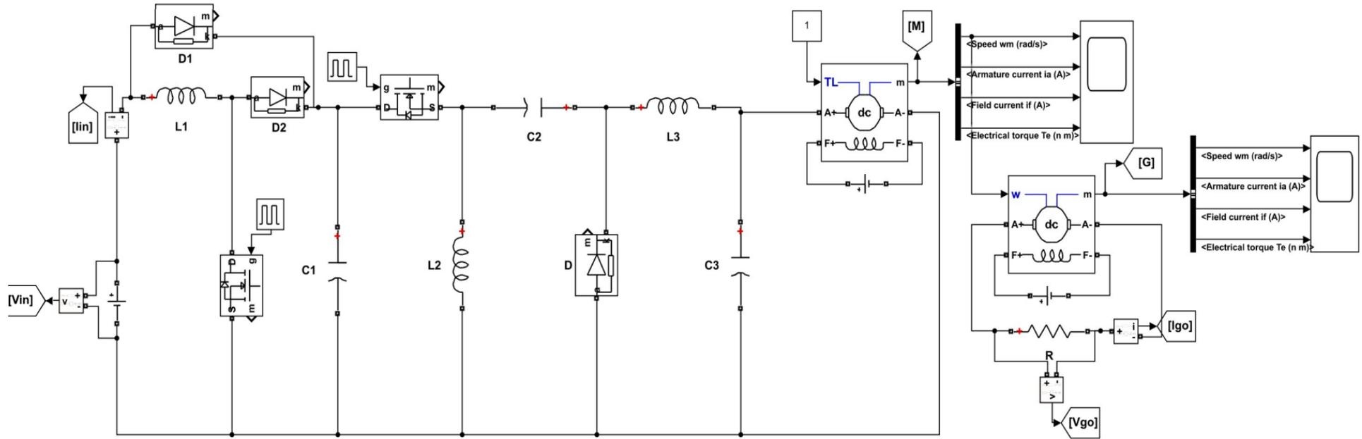
Figure 6. Simulation model of Zeta converter-fed Separately excited DC motor coupled with DC generator
