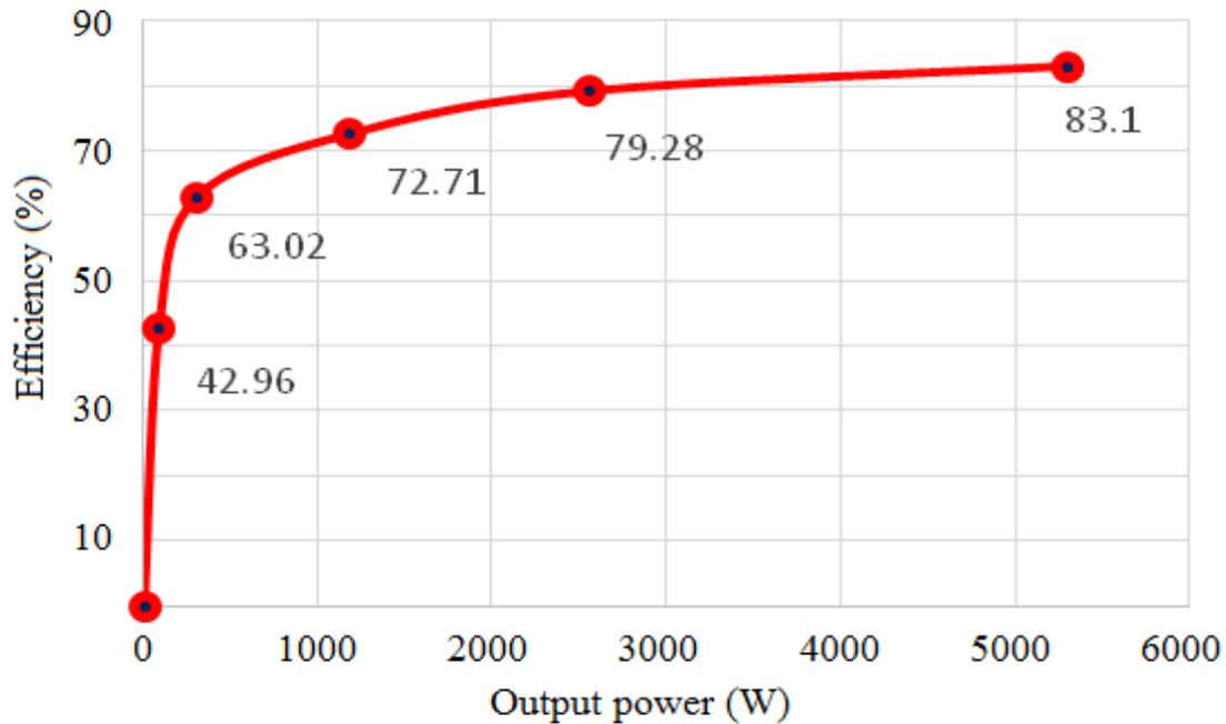
Figure 15. Efficiency characteristic of motor-generator set
