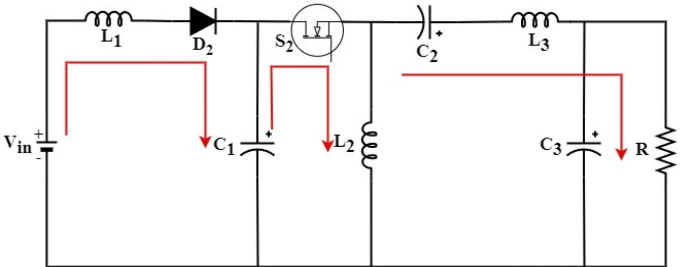
Figure 4. Equivalent circuit of the converter during Mode-III
