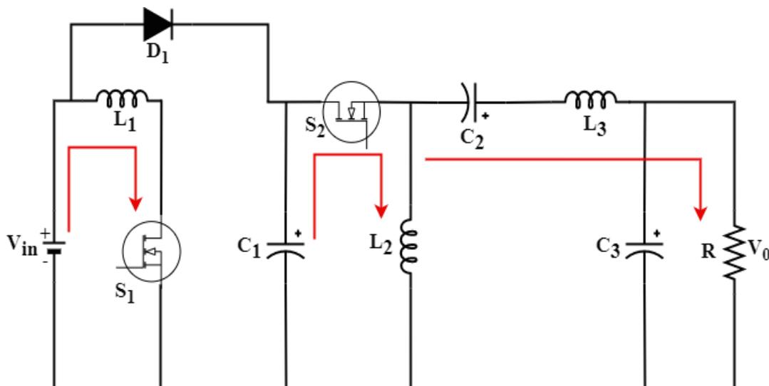
**Figure 2.** Equivalent circuit of the converter during Mode-I
