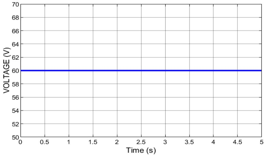
**Figure 8.** Converter Input voltage (V<sub>in</sub>)
