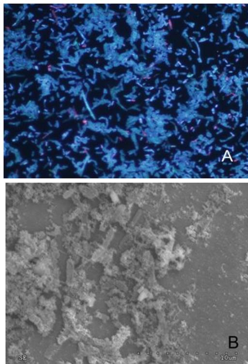
**Figure 1** - Observation of biofilm with the use of fluorescence microscope Olympus GX71(A) and scanning electron microscope HITACHI S-3000N (B).
