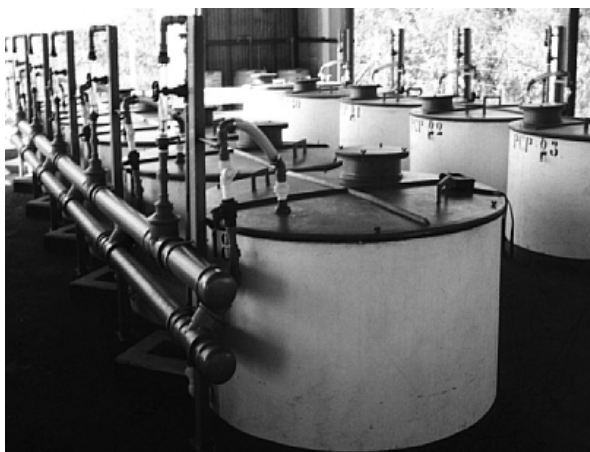
Figure 1 - Bioreactors with a capacity of 400 kg soil used for fungal culture, São Vicente, SP (Photo: Ricardo R. da Silva, 2004).
