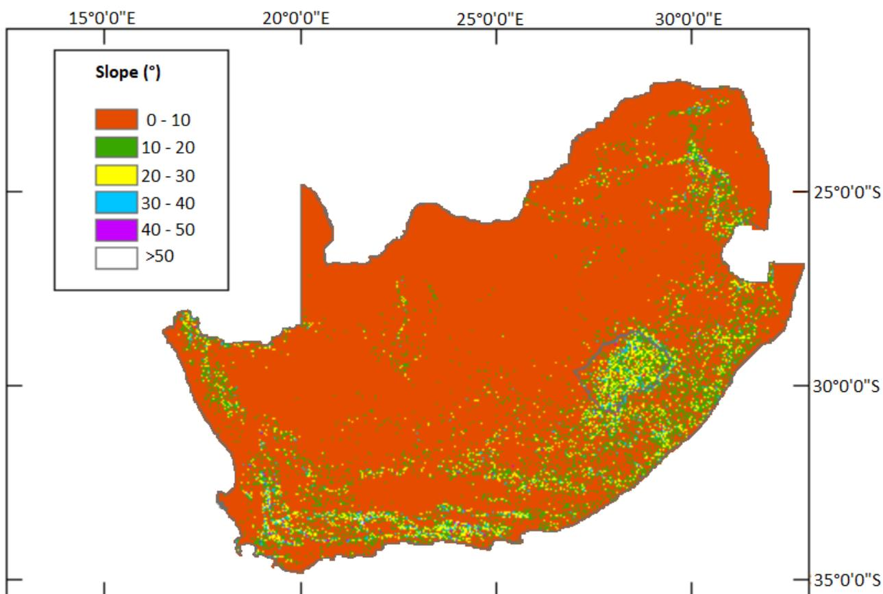
Figure 3: Categorized slope representation over South Africa based on SRTM data (units are in angular degrees).
