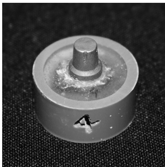
Figure 1. Metal cores included in PVC rings.
