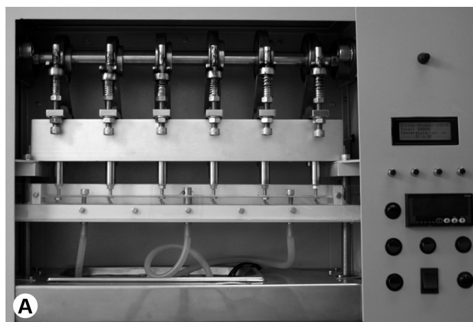
Figure 1. A. Mechanical cycling machine; B. Sample submitted to mechanical cycling.
