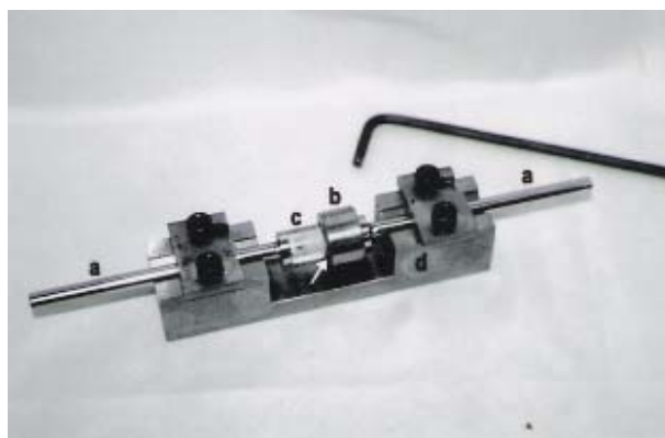
Figure 1. Tensile bond strength apparatus. (a) = pair of metal rods; (b) = circular metal matrix including the enamel surface; (c) = transparent acrylic cylinder containing the composite resin; (d) = alignment block; Arrow = adhesive interface.
