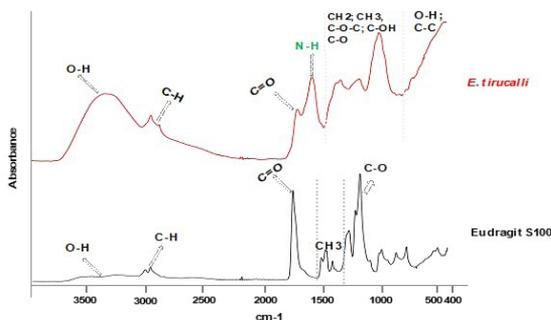
**Figure 2.** Comparative infrared spectrum of the extract and eudragit S100.
