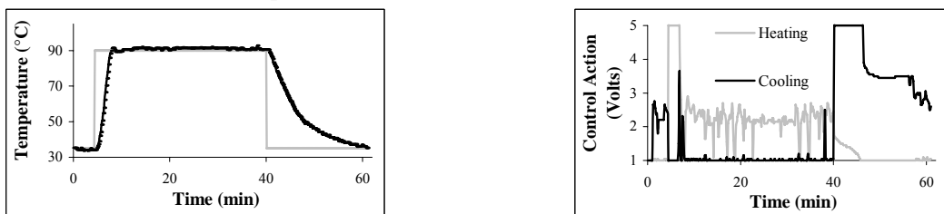
Figure 7: Temperature behavior and actuators action ( \alpha=0.50 ; \lambda_c=0.1 ).
