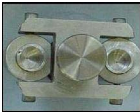
Figure 2: Aluminum tubes installed on the head of the MA – 860 microcentrifuge.
