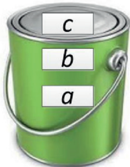
Figure 1. Sketch of the simulated system: a) liquid paint phase; b) air and vapor phase; c) condensed phase.
