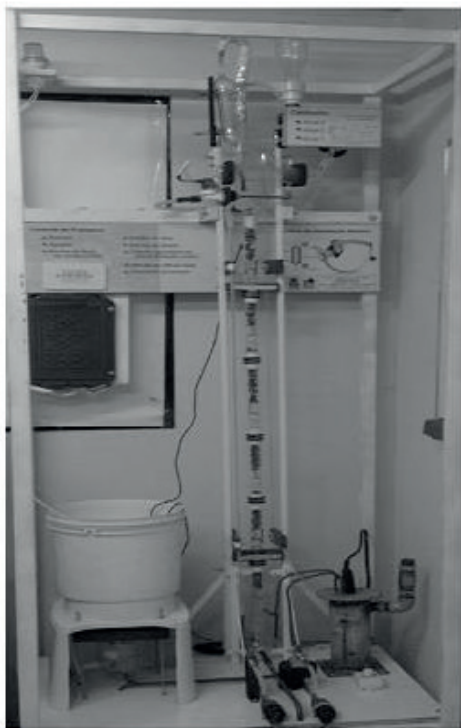
Figure 2. Reactive Distillation Column for biodiesel production process.
