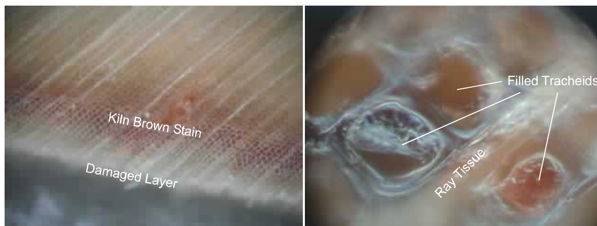
Figure 2: Light micrographs of the kiln brown stain layer viewed on a transverse section.
