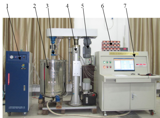
1. Steam generator 2. Stirred tank 3. Torque meter 4. Hydraulic lift device 5. Speed drive unit 6. Temperature control instrument 7. Control cabinet.
