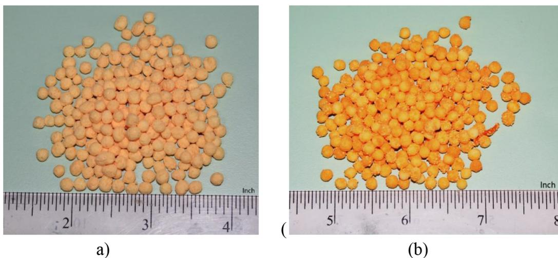
**Figure 4.** Photographic view of (a) St-PCU with uniform coating and (b) St-PCU with distorted coating layer having dried solid particles on the surface.
