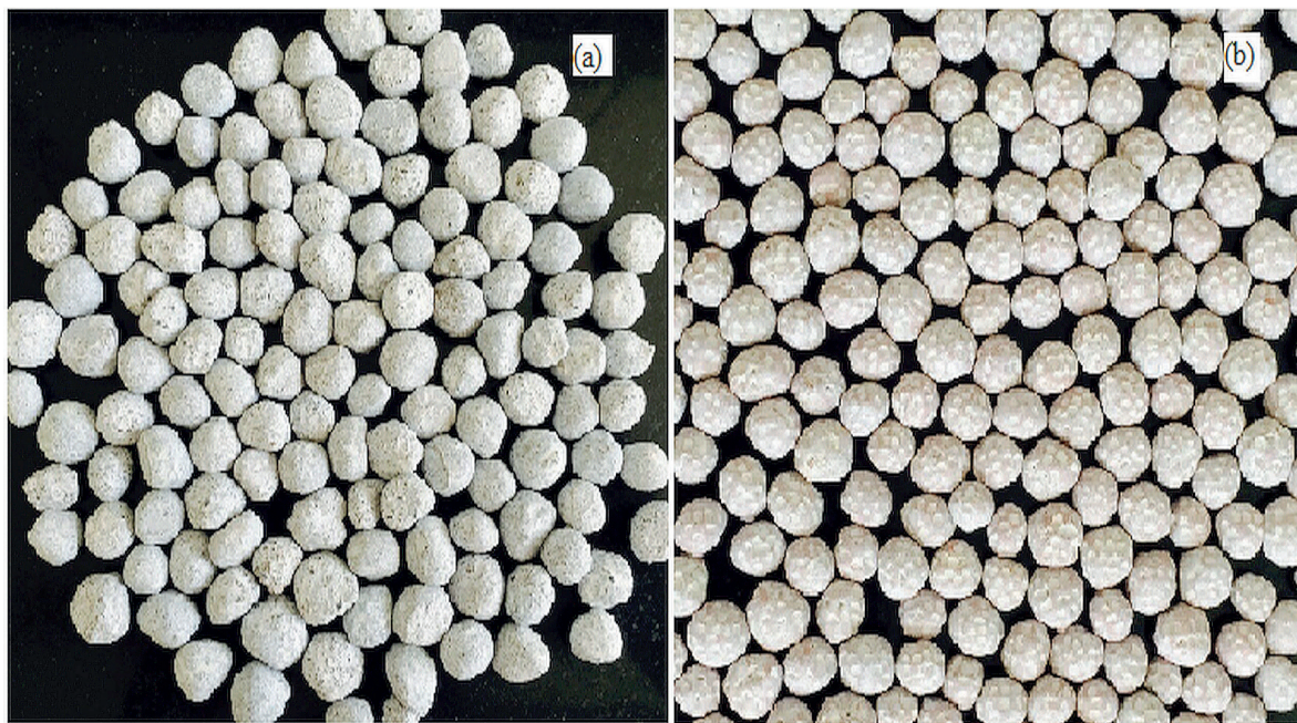
Figure 1. (a) TiO 2 coated cement beads and (b) TiO 2 coated clay beads.
