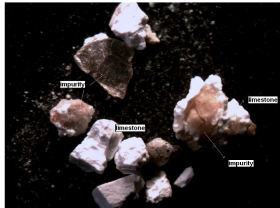
Figure 3: Optical micrograph of limestone Cd showing the presence of impurities.
