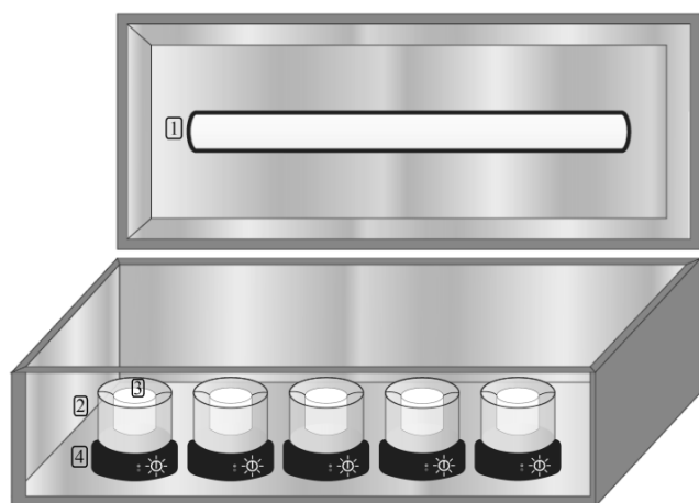
Figure 1. Photocatalytic bench reactor model. 1. Germicidal lamp (2,500 lux and 18.6 µW.cm -2 at 254 nm); 2. Glass reactor; 3. Metal plate with immobilized TiO 2 ; 4. Magnetic stirrer.
