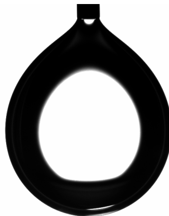
Figure 1: Image captured by the OCA 15E tensiometer for measuring the interfacial tension of the water-cyclohexane system. A needle with an outer diameter of 0.714 mm was used.
