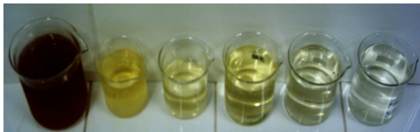
Figure 6: Effect of the variation of the current density (from left to right - raw effluent; treated effluent with iron electrode with 25; 50; 75; 100 and 125 A/m^2 , respectively).
