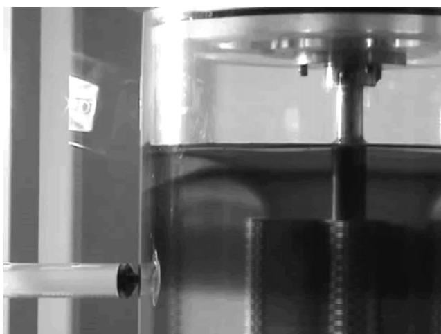
Figure 4: Injection of the tracer fluid into the vessel and formation of the vortex above the impeller.
