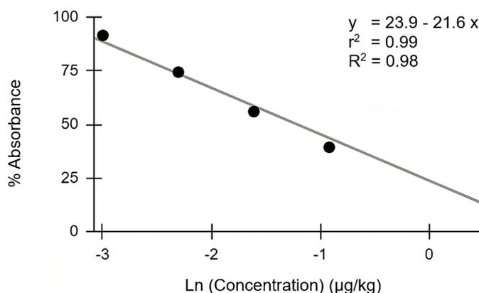
**Figure 1.** Standard curve of microcystin in linear form.
