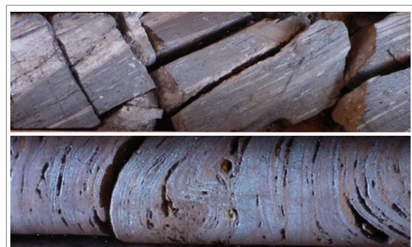
Figure 16. Above, fresh iron formation constituted by bands of magnetite, quartz and silicates. Below, weathered, with layers of martite and hematite replacing magnetite, and with limonite replacing silicates and most of the quartz. The texture of the bands varies from massive to friable. Open spaces indicate where minerals were completely leached out.
