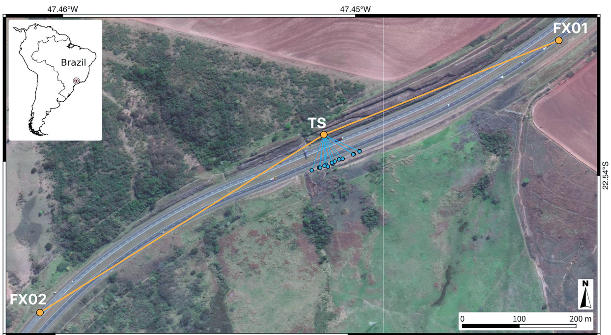
Figure 1. Study area location in Brazil (inset). Positioning of the total station (TS), fixed points (FX01 and FX02) and targets distributed on the outcrop surface (blue points).
