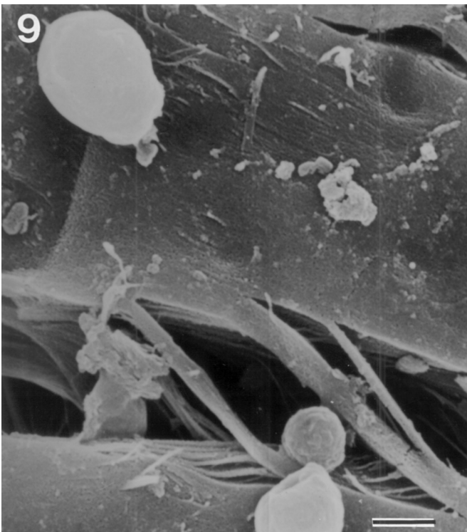
Figure 9. Growth of yeast cells on the upper surface of membrane (#245 route) (Bar = 2 nm).
