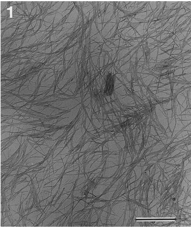
Figure 1. Fibrils of pseudoboehmite (Bar = 250 nm).
