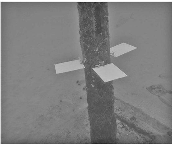
Figure 2. Biofouling multi-experimental units used in the present study to support the PVC panels.
