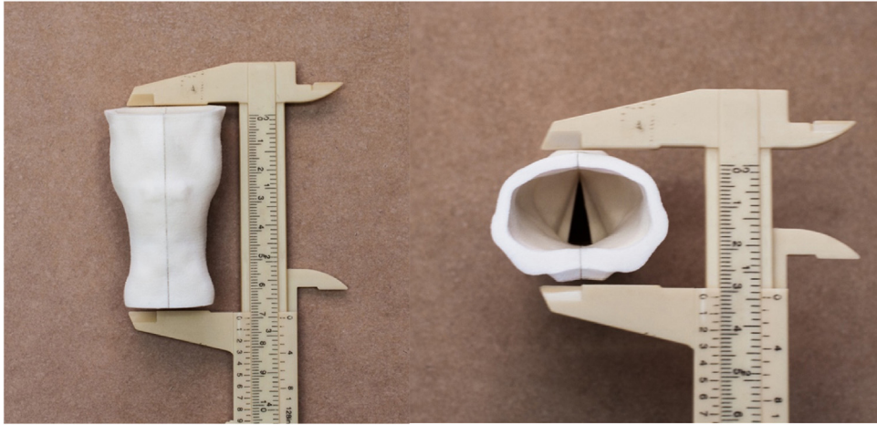
Figure 1 (Left) Images of the anterior aspect of the model measured in centimeters. (Right) Image of the superior plane of the larynx printed in 3D, measured in centimeters. Source: the author.
