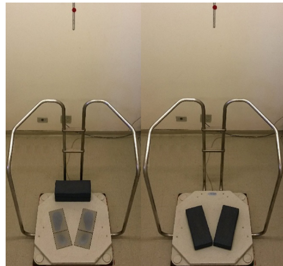
Figura 1 Equipamento do Tetrax Interactive Balance System (Tetrax IBS™).
