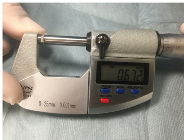
Figure 1 Measurement of the thickness of tragal cartilage using a micrometer.
