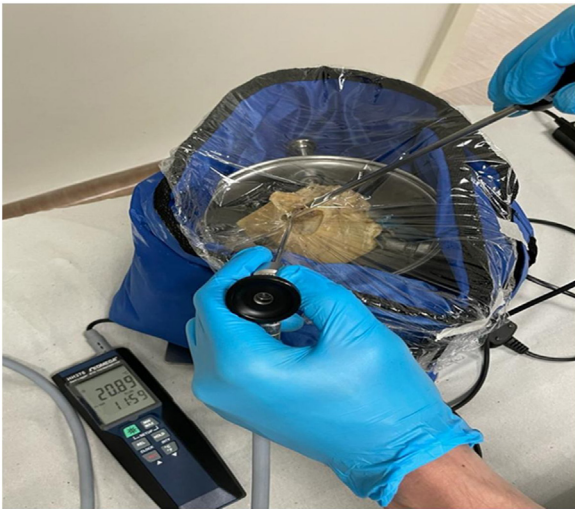
Figure 3 Endoscope and thermometer inserted into the temporal bone through the perforations made in the PVC plastic film.
