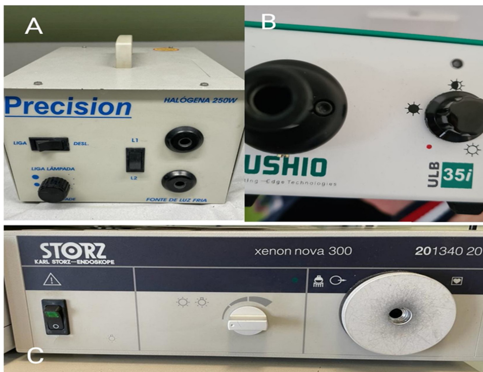
Figure 1 Light sources used. (A) Halogen. (B) Light Emitting Diode (LED). (C) Xenon.
