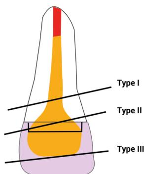
**Figure 3.** Failure pattern of the specimens according to the type of fracture (I- Catastrophic fracture of the crown and/or remnant (below CEJ); II- Fracture of the crown with remnant above or at CEJ; III- Debonding of the glass-ceramic crown).
