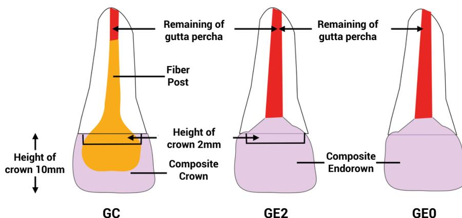
**Figure 1.** Image of the section type according to the amount of wear. GC - Control group; GE2 – endocrown with 2 mm ferrule group; GEO – endocrown with 0 mm ferrule group.
