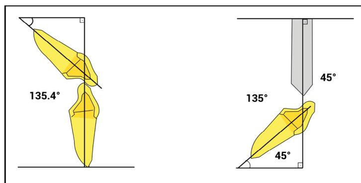
**Figure 2.** Schematic drawing of test specimens subjected to load at 45° in a universal testing machine. Pressure from the rod tip was applied at a crosshead speed of 1 mm/min (3 mm below the incisal edge) on the palatal surface of the crown.
