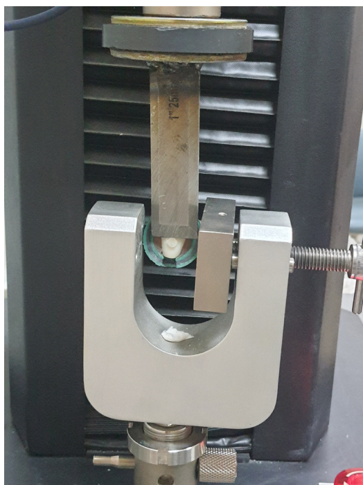
Figure 3. Universal machine loaded with specimen, the blade is parallel to the adhesive interface
