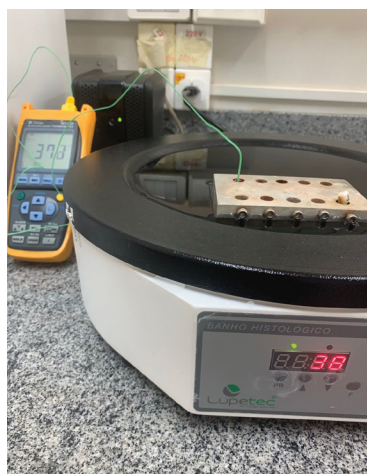
Figure 1. Tooth remained fixed in a metallic structure immersed in a water bath at a temperature of 37°C with water up to the cervical region.
