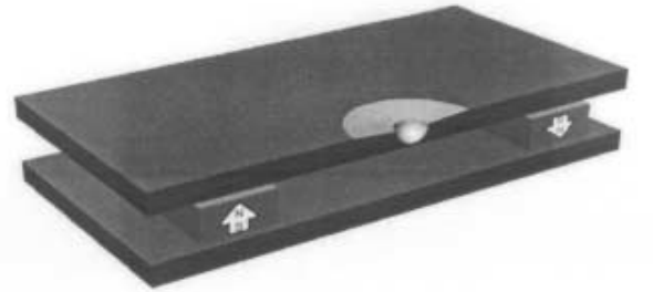
Figure 7. Schematic drawing of half the magnetic circuit used to test the inverse technique. NdFeB magnets with opposite orientations join the two plates. The magnetic field sensor is not shown.
