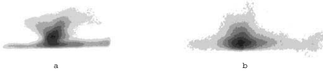
Figure 6. Time integrated pinhole images of soft X-ray emission from (a) deuterium (b) deuterium-krypton admixture.
