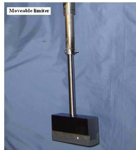
FIG. 1: A photo of moveable limiter with graphite tip.
