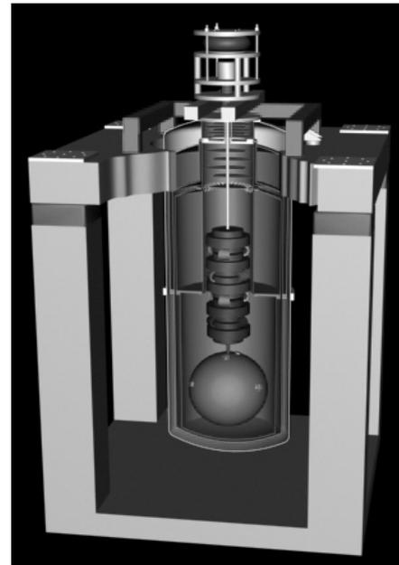
FIG. 3: Schematics of the SCHENBERG gravitational wave detector.
