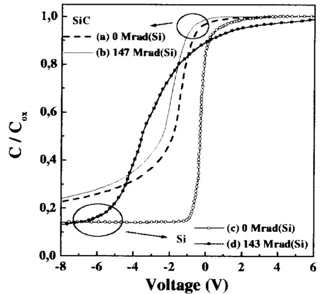
Figure 2. Capacitance-voltage characteristics of a Si MOS and a SiC MOS capacitor irradiated with similar x-ray doses.
