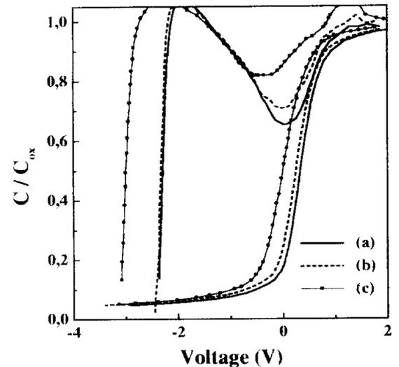
Figure 3. Capacitance-voltage curves of a 6H-SiC MOS capacitor exposed to different x-ray doses. Oxide thickness is  $9\text{ nm}$  and gate area is  $7.85 \times 10^{-3}\text{ cm}^2$ . Doses in Mrad(Si) are: (a) 0, (b) 14, (c) 110.
