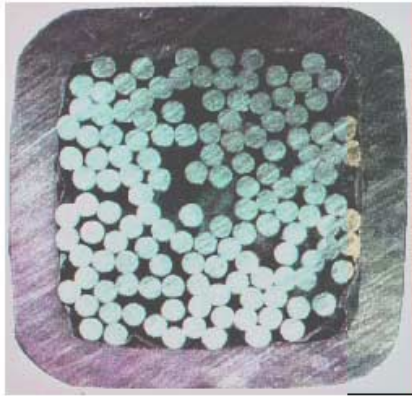
Figure 2. A cross sectional view of SST-1 CICC with 135 strands in it.
