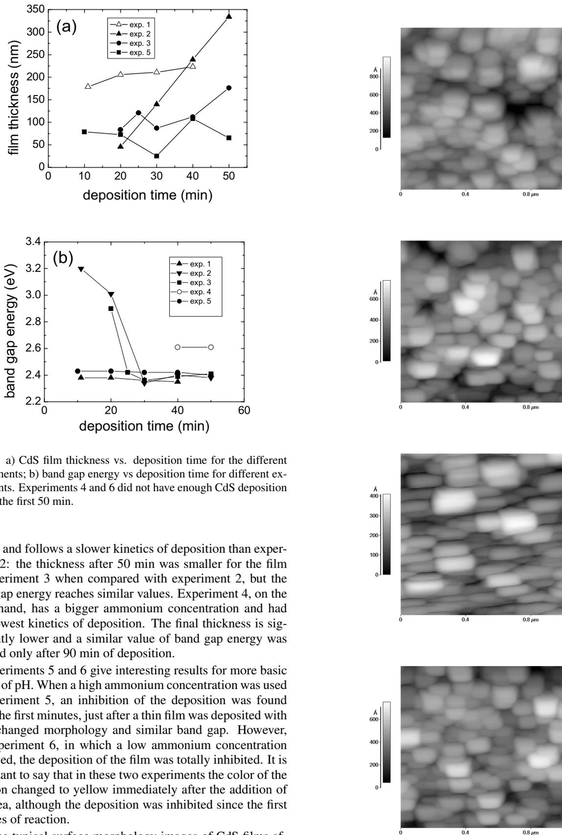
FIG. 2: a) CdS film thickness vs. deposition time for the different experiments; b) band gap energy vs deposition time for different experiments. Experiments 4 and 6 did not have enough CdS deposition during the first 50 min.
