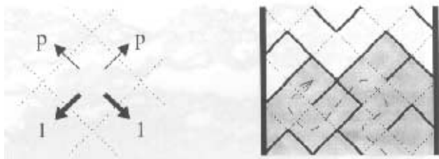
Figure 4. Simple model exhibiting a depinning transition. The pores are represented by cells on a diagonal square lattice. The permeability across the edges of the cells depends on the direction of flow: In the downwards direction all edges are permeable whereas in the upwards direction they are permeable with probability p and impermeable otherwise. The right panel of the figure shows a particular configuration of open (dashed) and closed (solid) edges. Pumping in water from below, the interface becomes pinned along a directed path of solid lines, leading to a finite cluster of wet cells (shaded region). The dashed arrow represents an open path in order to illustrate the flow.
