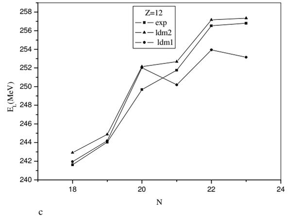
FIG. 1: Representation of experimental and calculated binding energies using the two liquid-drop models (ldm1 [1] and ldm2) versus  $N$ . a)- Ne isotopes, b)- Na isotopes, c)- Mg isotopes.
