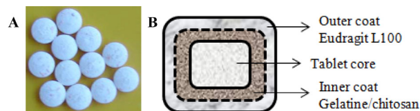
FIGURE 1 - Bilayer coated tablet. Bilayer coated tablet was prepared in this study (A); schematic of the bilayer coated tablet delivery system (not to scale) (B).
