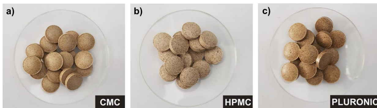
FIGURE 1 - Visual aspects of tablets containing Carboxymethylcellulose (a), Hydroxypropylmethylcellulose (b), and Pluronic (c).
