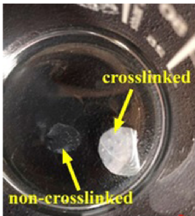
FIGURE 2 - Naftifine-loaded NFT/PVA/SA and GTA/NFT/PVA/SA nanofiber mats after immersing in water for 24 h.
