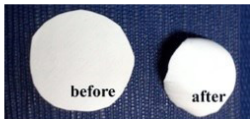
FIGURE 1 - Naftifine-loaded PVA/SA nanofiber mats before and after the crosslinking procedure.
