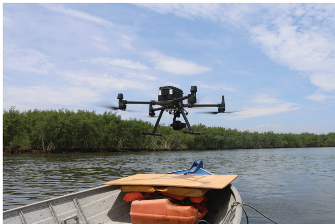
Figure 2. TOPODRONE 200 Ultra embedded in FJI M300 RTK drone, the profiler includes a Velodyne Ultra Puck sensor, a high-precision IMU (Honeywell), and a receiver HNSS L1/L2 Survey (U-BÇOX).
