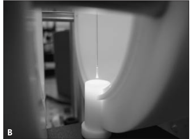
Figure 2 A and B - Positioning of the sample port and optical fiber inside the Teflon sphere in the reflectance analysis set.
