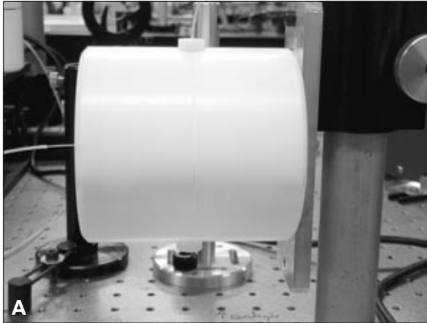
Figure 2 A and B - Positioning of the sample port and optical fiber inside the Teflon sphere in the reflectance analysis set.
