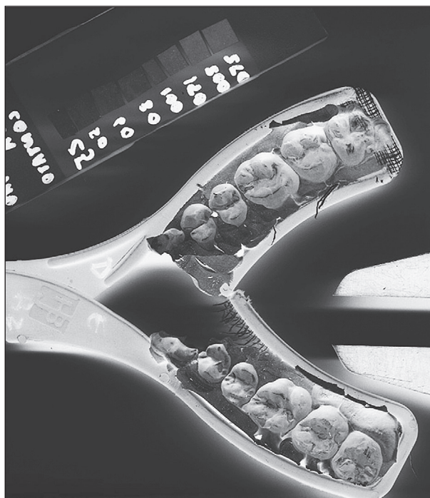
Figure 2 - Transformed to grayscale and inverted image of silicon record used to establish silicon thickness.
