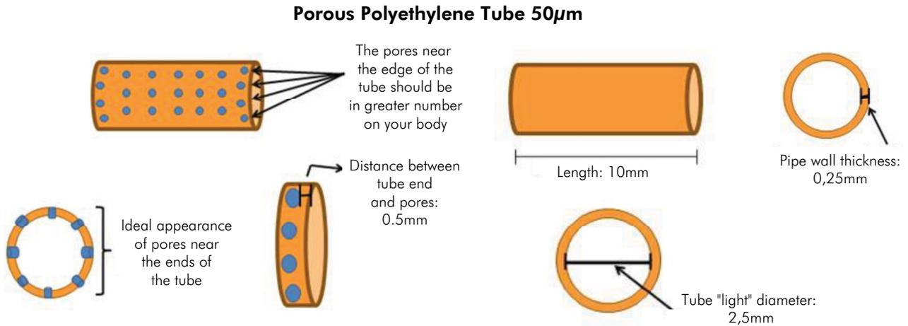
**Figure 2.** Schematic demonstration of the porous polyethylene tube.
